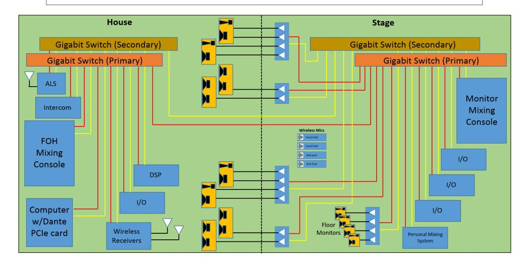
**System Description:** This is a block diagram for a medium to large size House of Worship or Performing Arts Center. The house and stage systems are running on a redundant Dante network. All devices shown are Dante enabled with the exception of the loudspeakers, which are driven by Dante-enabled amplifiers.
