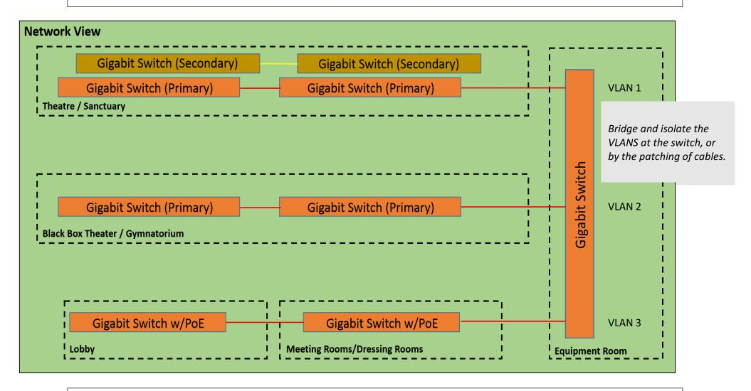
**System Description:** The network view of the system shows all of the switches that are part of the Dante network connection to a single central switch. The switch can be configured to allow the system to act as one large system, or isolate the individual systems.
