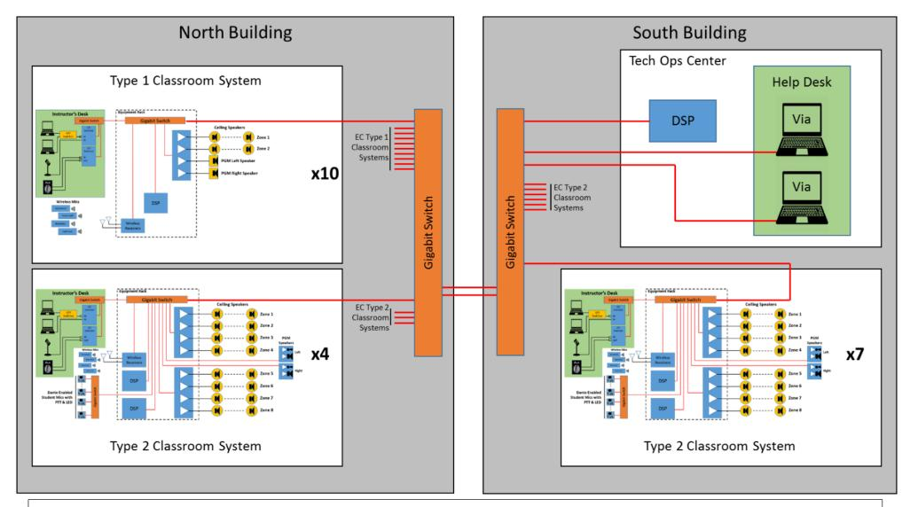
**System Description:** This is an overview of the facility show two buildings, with the North Building contain 10 of the small and 4 of the large audio systems. The South Building has 7 of the large audio systems with a Technical Operations Center and Help Desk which are using Dante Via to both listen and communicate with the rooms.
