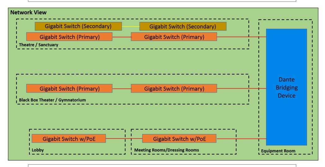
**System Description:** The network view shows a Dante enabled bridging device that can be used not only to isolate the three systems, but makes it easy to route various audio channels between the systems, while providing full isolation (and sample rate conversion). A bridging device is any product that can host multiple Dante I/O cards while providing sample rate conversion, such as a mixer or dedicated format convertor.
