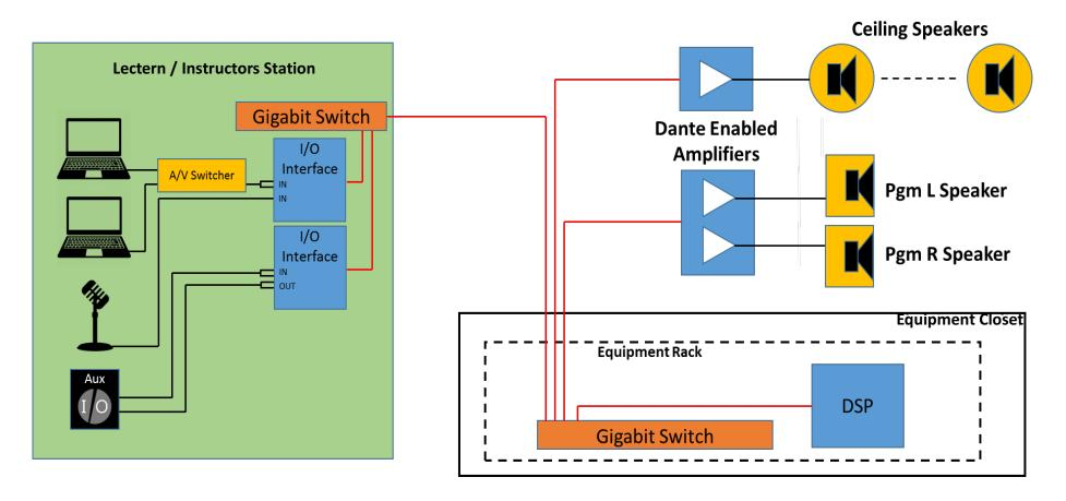
**System Description:** This diagram is what a typical presentation or training room audio system can look like using Dante. The lectern or instructors station can use Dante I/O devices which connect to the DSP located in an equipment closet. The amplifiers are remotely located in this example, but they could just as easily be colocated with the DSP in the equipment rack.
