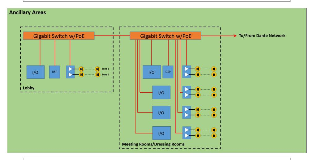
**System Description:** This diagram shows the ancillary areas of the facility, including the lobby and meeting rooms and/or dressing rooms. PoE Gigabit switches are used since the design utilizes many low channel count Dante I/O devices that can derive power directly from their Ethernet connections.
