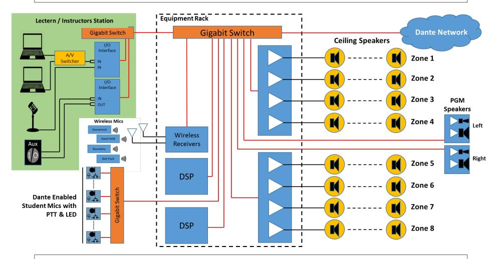
**System Description:** This system replaces the analog microphones with Dante enabled ones. It simplifies the wiring and any related infrastructure costs.
