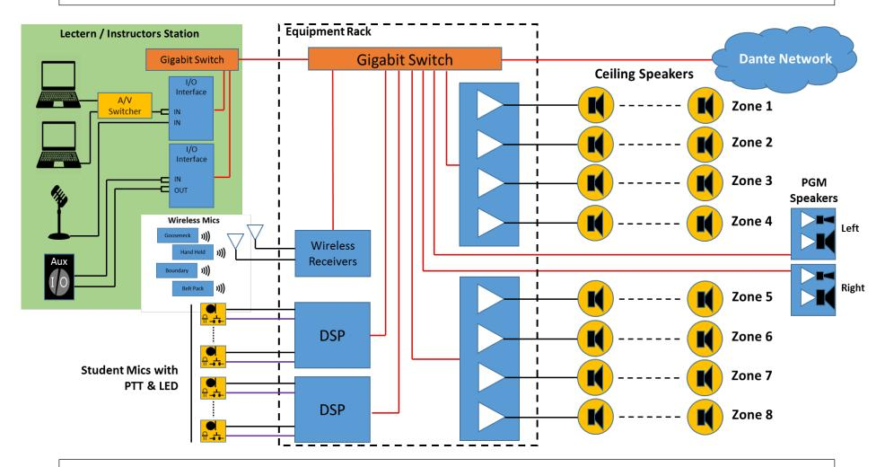
**System Description:** This system design builds off of the previous one by adding more microphones (both wired and wireless) for the meeting participants or students. Additional DSPs are used and the analog microphones used have PTT logic and LED status indicators which are wired to the control ports of their respective DSPs. A mix-minus speech reinforcement system is added along with Dante enabled program audio speakers.
