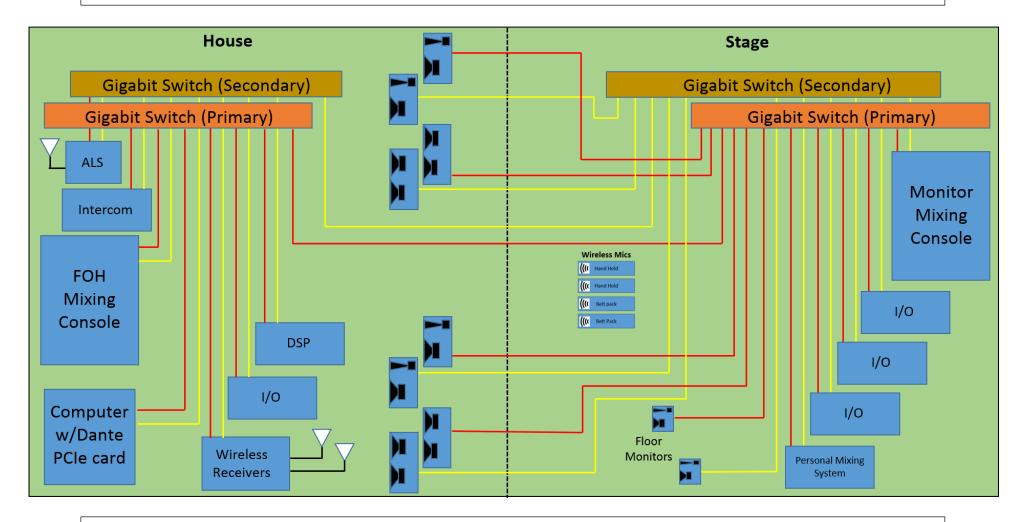
**System Description:** This block diagram shows the same system, but now has Dante enabled loudspeakers for both the front-of-house and the stage monitors.
