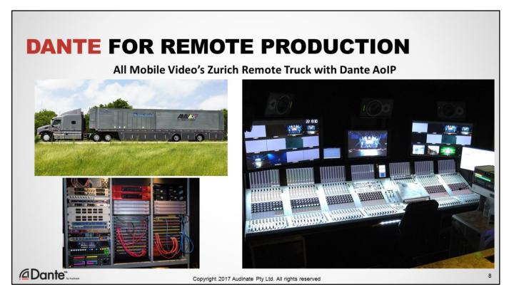
All Mobile Video (AMV) debuted a new remote truck in late February 2016 at iHeartRadio's inaugural iHeart80s Party in Los Angeles with 11 Focusrite RedNet converters installed to handle management and distribution of the audio communications, IFB and camera control circuits throughout the video and audio production environment.
