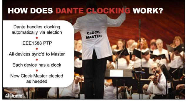
While several adjustments are permitted, the important thing to know is that by default, Dante handles clocking 100% automatically. If you did nothing to adjust clocking on a Dante system, it will work perfectly. Only external clocks require any configuration to work.
